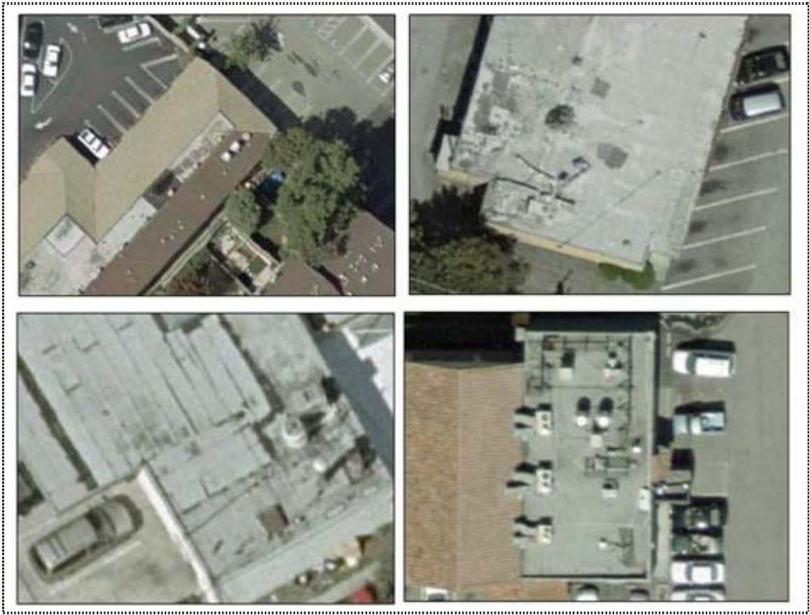
Figure 8 – Example Dry Cleaner Roof Vent Features from High Resolution Aerial Photos
